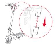
Secure the handlebar and stem assembly with the supplied screws and tighten the screws with the included wrench. Recommended torque is 4Nm to 5Nm.
