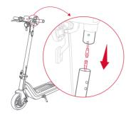
Secure the handlebar and stem assembly with the supplied screws and tighten the screws with the included wrench. Recommended torque is 4Nm to 5Nm.
